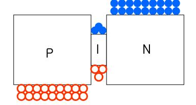
Injected carriers are spread-out => smaller density
