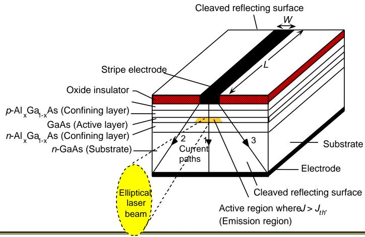
Efficient carrier confinement: PIN structure with large  $E_g$  for P, N regions
